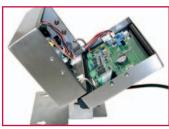
Internal Hinge Mechanism Easy access for option installation and servicing
