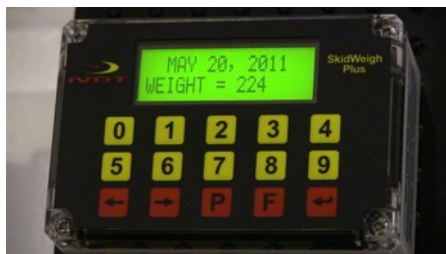
ED3-SM Standard LED display check weighing with visual / audio warning to the operator.
