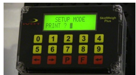
ED3-AT Standard LED display check weighing with accumulative load weight total.
