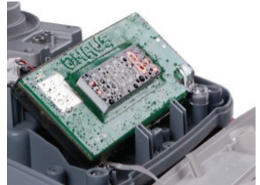
Inside PCBA Silicon Glue Sealing
