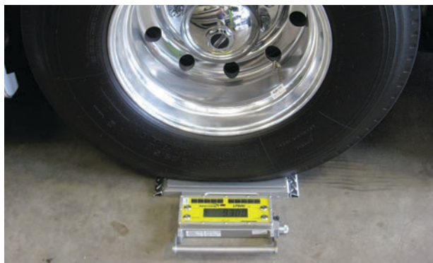
All LP600™ pads can utilize RFX™ Wireless Weighing to display individual axle weights and GVW on a variety of remote devices.
