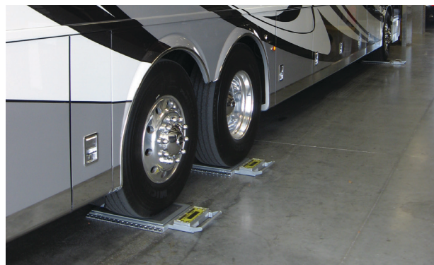
Individual wheel weights, axle weights and GVW (Gross Vehicle Weight) can be determined using an LP600™ scale pad under each wheel.
